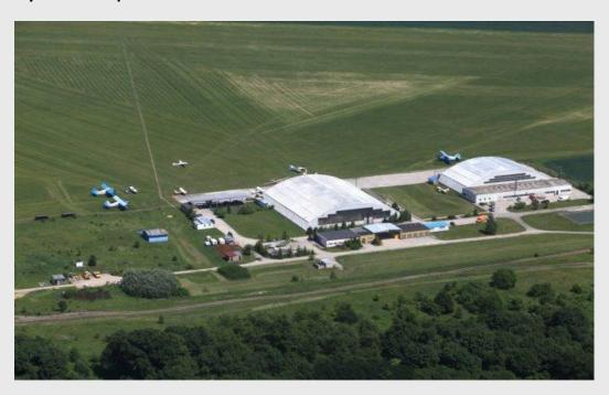
Szymanów Airport is home to the Wrocław sports Aeroclub, located in Szymanów 11 km from the city centre. The landing area has two grass runways: in the direction 14/32 with dimensions of 770 m x150 m and in the direction 12/30 with dimensions of 630 m x100 m.
