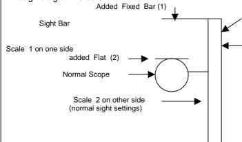
The technique used is that on first addressing the target he draws up several times and between each "draw" he moves the sight until the added fixed bar (1) is placed on the top of the target, and the flat (2) is on the bottom. He has a scale (Scale 1) pre-calculated so that in the above situation he can read off the distance to the target. Having "range found", he then sets his sight to the appropriate range (Scale 2) and takes his shot.
